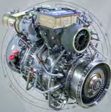
TEI-TS1400 Turboşaft Motoru
